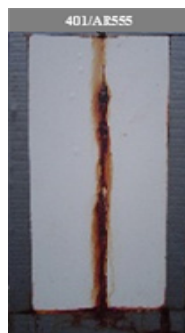
Salt spray after 750 hours exposure
