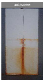
Immersion in NaCl 3.5% after 750 hours exposure
