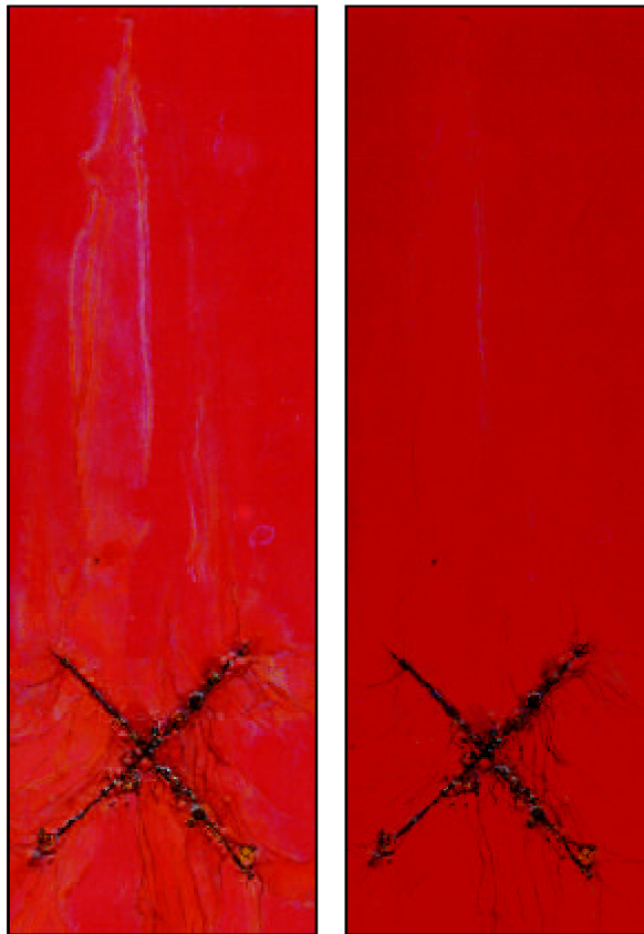
Beckopox primers above, show 1500 hours salt fog results with 2 mils on phosphated steel. The formulation on the left contains 1.4% Benzyl Alcohol. Total VOC is 1.51 pounds per gallon.
